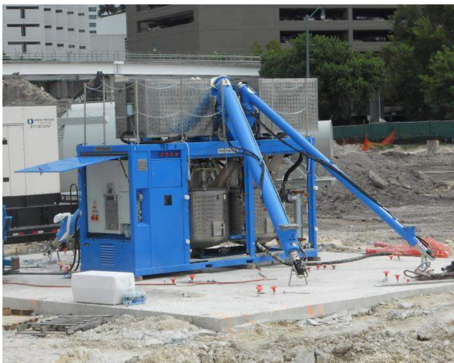
Mixing plant OM 1000/2-48 with hydraulically driven charging augers
